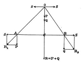
At A and B apply two equal and opposite forces S, S
